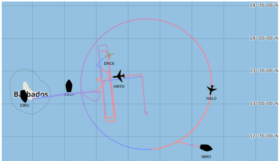
Flight A: ATR (HMT0) trajectory. The shift in rectangles and L-patterns shows the INS problem on the ATR, that will have to be post-processed. The actual trajectory was sticking on the same tracks for both patterns.
