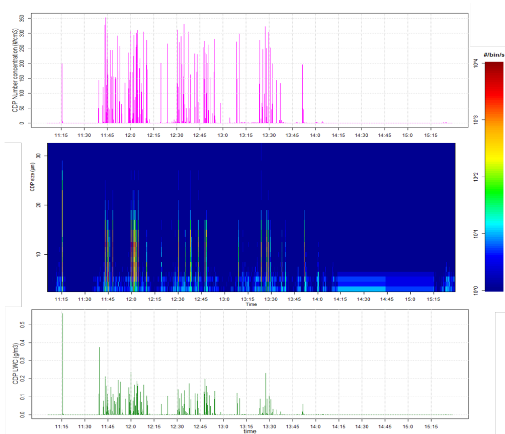
Quick look of microphysical measurements: Time evolution of (Top) cloud droplet number concentration [ \text{cm}^{-3} ], (middle) cloud droplet sizes [microns] and (bottom) liquid water path [ \text{g/m}^3 ]. Courtesy Alfons Schwarzenboeck.
