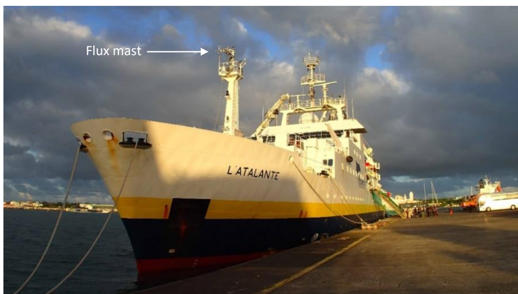
Figure 1. The R/V Atalante and the flux mast on the meteorological tower of the front deck
